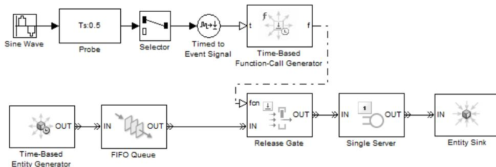
In this model, the **Event generation mode** parameter of the Time-Based Function-Call Generator block is set to **Period** from port. The Probe block detects the sample time of a sine wave signal and connects it to the input port **t** of the Time-Based Function-Call Generator block. The value at the input port **t** determines the period — or time delay — between successive function-call events generated by the block and is used to control entity advancement through the Release Gate block.
