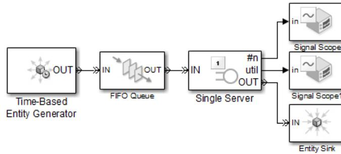
The server has idle periods that reduce its utilization. However, the server block recomputes the **util** signal only when the number of entities in the server changes. While the definition of utilization says that the utilization is less than 1 at time 3, the **util** signal remains at its previous value of 1 until the next entity arrives at time 4.
