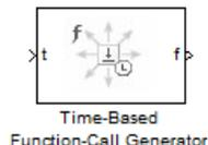
This block generates function-call events, either once at the start of simulation, using an intergeneration period that you specify in the block dialog box, or using a signal connected to the input port. The intergeneration period is the time interval between two successive generation events.
